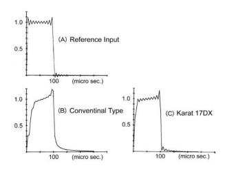
In summary: The adoption of the KARAT series 1.7mm long solid diamond cantilever was the result of proven research and development providing the least disturbed waveform and fastest transmission speed between the high and low frequencies up to 100KHz. The absence of any hardness particularly in the important high frequency area is immediately distinguished, providing both articulate and delicate reproduction of analog recordings with no hint of a loss of bass.
