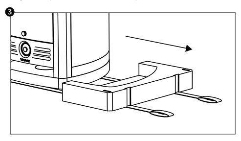
**Vintage Ten:** lift the loudspeaker off the foam end cushions and fit the 4 floor coupling spikes and locking wheels. When the loudspeaker is in position, level by adjusting the spikes and tighten the locking wheels (Fig. 4).
